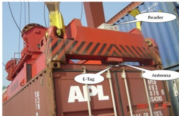
Figure 5 Reader and antenna fixed on gantry crane
